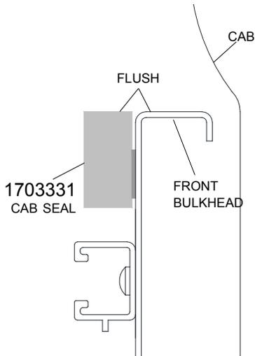
**STEP 2A:** Apply additional bulkhead seal provided directly underneath of the factory bulkhead seal on the front header, trim ends flush. **STEP 2B:** Position cab header over front bulkhead and cab seal as shown below. Install your tonneau cover as shown in owner's manual.
