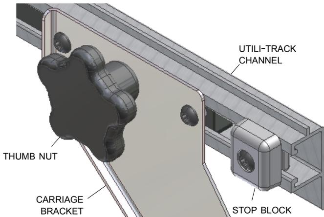
**STEP 3:** Install Spacers: Disassemble carriage brackets. Re-assemble as shown.
