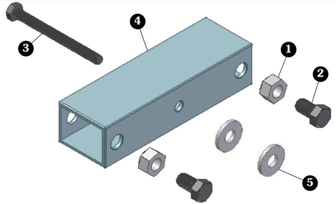
**STEP 1:** Adjust Width of Bed Extender Cage: Open tailgate and remove bed extender cage. Measure and record width of cage. Using a #20 torx wrench, loosen torx bolts from wedges. Pry wedges loose and slide tubes together, so that cage is 4" narrower than it was originally. Replace wedges and retighten torx bolts.
