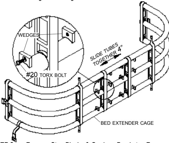
**STEP 2:** Remove Stop Blocks & Carriage Brackets: Remove stop blocks. Loosen thumb nut and remove carriage brackets from Utili-track channels.
