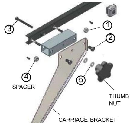
**STEP 4:** Replace Carriage Brackets: Slide carriage bracket assemblies into Utili-track channels. Re-install rear stop blocks and bed extender cage, following manufacturer's instructions.
