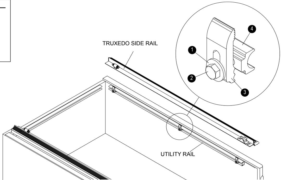
**STEP 1:** Insert clamp assemblies into utility rails, three on each side of pickup bed.
