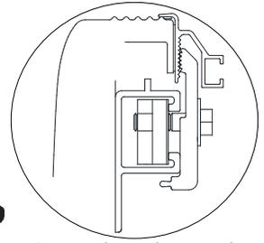
Picture above shows underbody rail correctly installed to track system.
