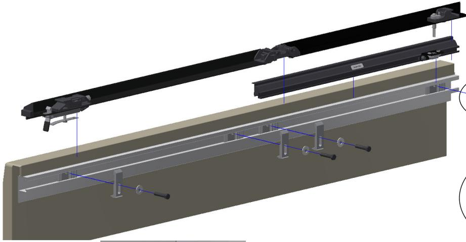
Clamp half 1703481 is installed in the Utility Track.
