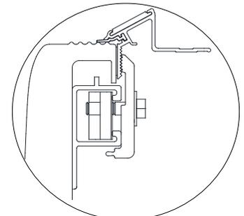
Picture above shows side rail correctly installed to track system.
